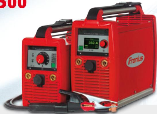
/ The TransPocket 2500/3500 units are the ideal appliances for using both out in the field and in production operations. Their light weight and standard carrying handle make them easily portable, while their robust design makes them shock-proof and just about indestructible. The higher-placed ventilation slots stop any water getting in, and the integral dust filter provides reliable protection against dirt.
